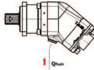
The motor casing flushing can be achieved by means of a flushing valve or directly from the return hose. Too low return pressure must be compensated by a back-pressure valve. The tank hose must be connected into the highest point as shown in the picture.
