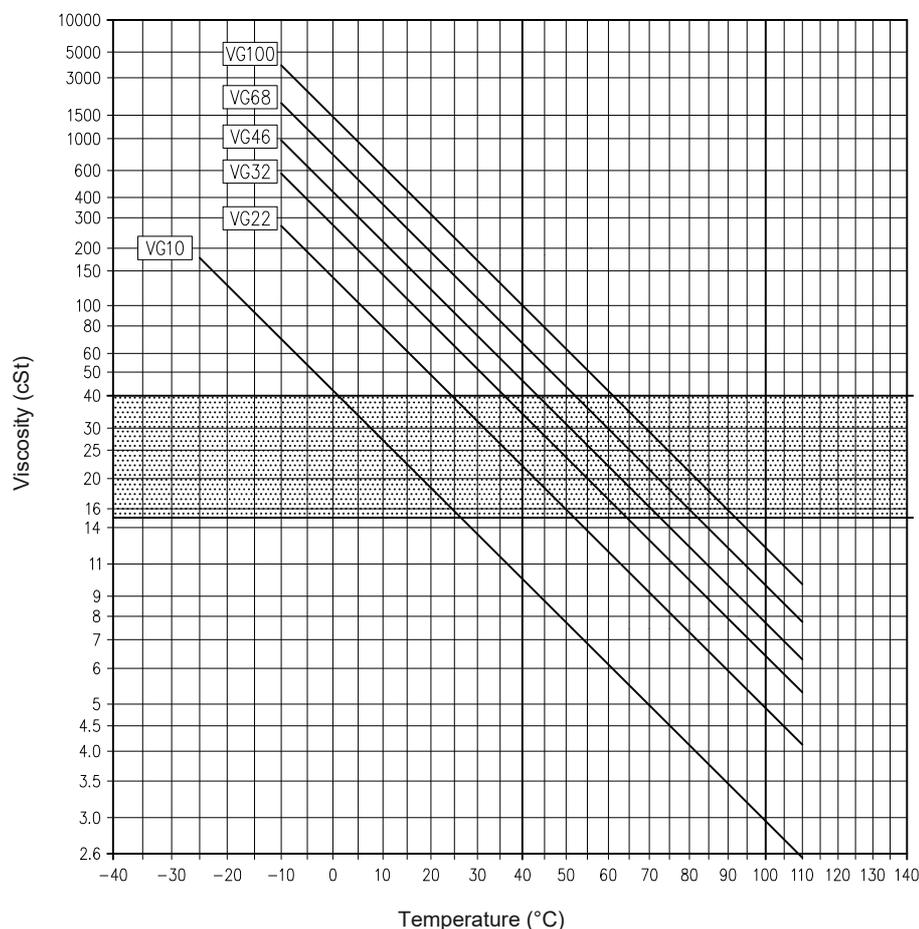
\* The diagram is only an example. It shows the viscosity temperature characteristics of typical fluids with different viscosities but sharing the same viscosity index. Ask to your hydraulic fluid supplier for the real viscosity-temperature diagram of the fluid used in your system.
