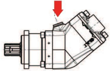
Connect the drain line before using the motor.
