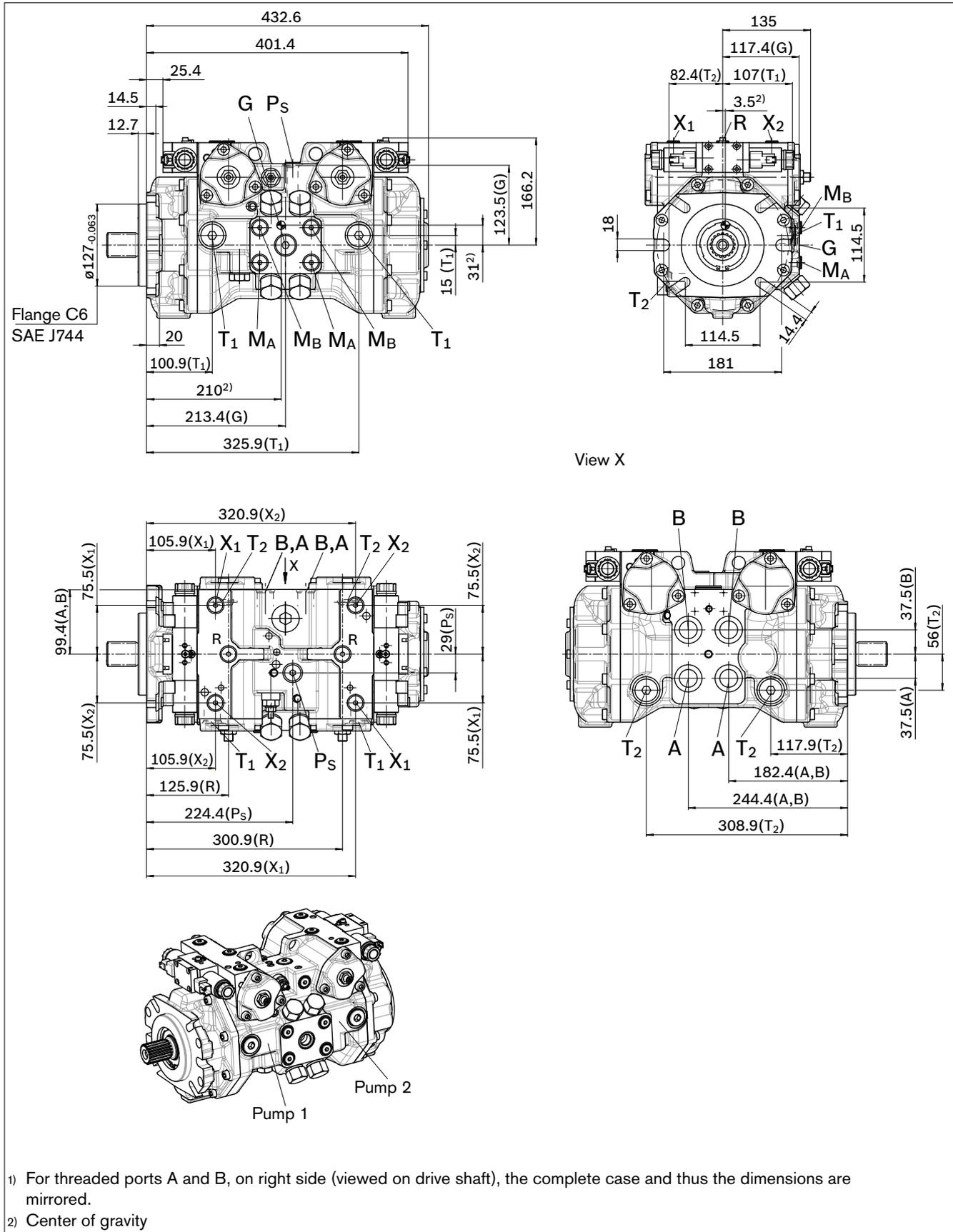
1) For threaded ports A and B, on right side (viewed on drive shaft), the complete case and thus the dimensions are mirrored.
